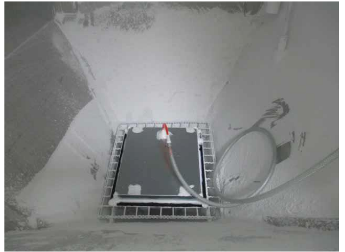
Before IP6X Test Photo
