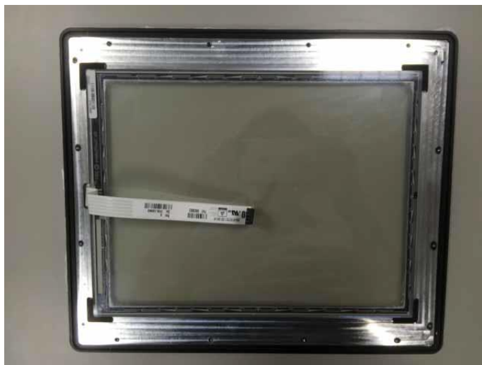
After IP6X Test Photo
